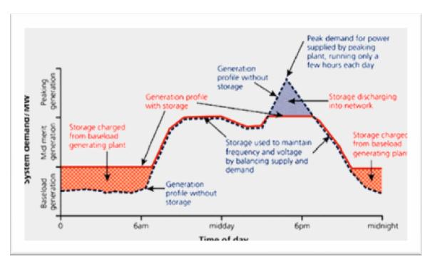
Figure 2.5: The role of grid connected storage (Electricity Storage Association, 2008)
