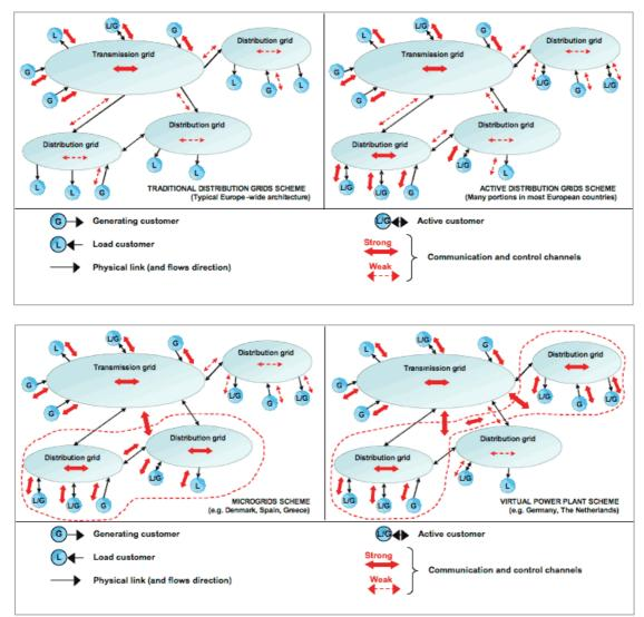
Figure 4.6: Various Distributed Generation Configurations (A. L'Abbate, G. Fulli, S.D. Peteves, 2008)
